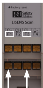
Connection contacts for a safety output 8k2
