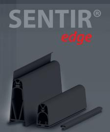
**SENTIR** *edge* safety contact edges are pressure-sensitive sensors for closing edge protection, with optimum overtravel distances and extremely fast switching behaviour. The Plug'n'Sense self-assembly system makes it possible to assemble a safety edge without tools or glue within a very short time and independent of ambient conditions, e.g. when servicing is required directly at the door. **Simple. Safe. Unique.**
